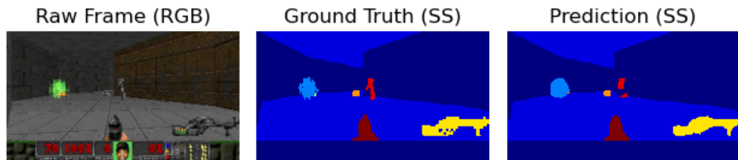
Figure 2.1: From left to right: an unprocessed RGB game frame from Doom; perfect semantic segmentation result; predicted semantic segmentation by DeepLabV3 model.
